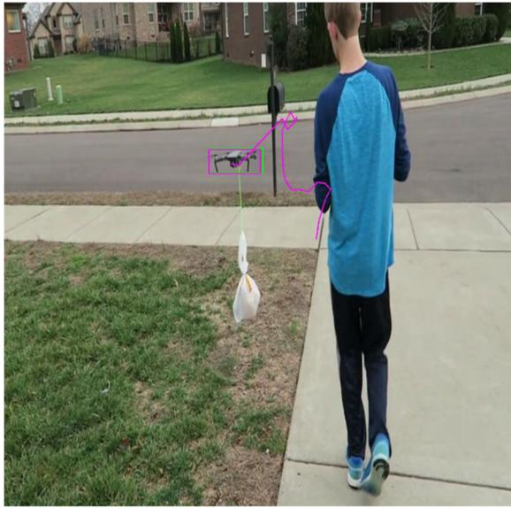
**Fig. 11** Performance of tracking. Lightweight YOLOv3 detector and TCT-based tracking perform well even with complex background
