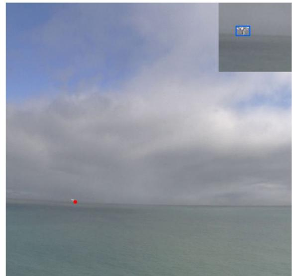
**Fig. 10** Detecting on multiple overlaid images. Simultaneous detection on a single overlaid frame composed of images coming from wide-angle camera and lowangle camera, with a single lightweight YOLO architecture. Also note that, even for very small sizes and difficult visibility conditions, the system can detect the drone on the horizon, while producing no false alarm [43]
