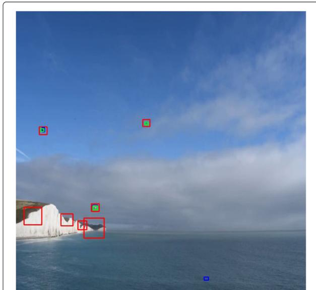
**Fig. 6** Comparison of detectors in a marine environment at far distance. Detections produced by lightweight YOLO architecture (green), cascaded Haar classifier (red) and Gaussian mixture model background subtractor (blue). There exists two birds, flying from left hand side toward right hand side on the upper half of the image and a drone approaching from horizon on the bottom half of the image, all three enclosed by green boxes. The footage is provided by [43]
