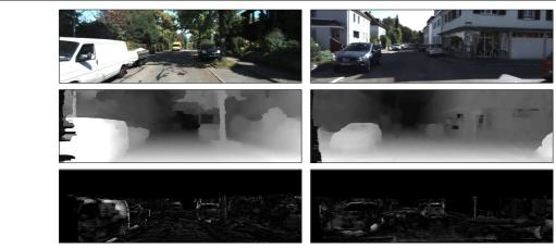
Fig. 8 Example results from the KITTI dataset. Top to bottom: left image, disparity map, and clamped disparity errors
